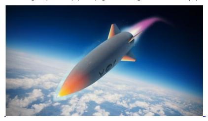
Launching from a B-52, the HAWC system's first stage boosted it to the targeted engine ignition envelope, where the Aerojet Rocketdyne scramjet engine fired and accelerated the system to speeds in excess of Mach 5. The system performed as predicted travelling more than 300 nautical miles and reaching altitudes above 60,000 feet.
