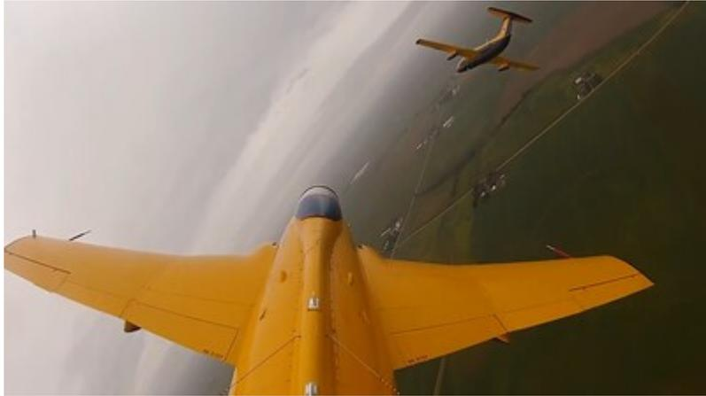
The successful flights are a significant milestone for Skunk Works' Tactical AI team, in which AI directly flew and conducted tactical exercises with a full-scale, live aircraft – one of OPL's L-29 Delfin jets – using heading, speed and altitude commands. The team executed simulated-to-real transfer test objectives against a virtual adversary in offensive and defensive risk postures.
